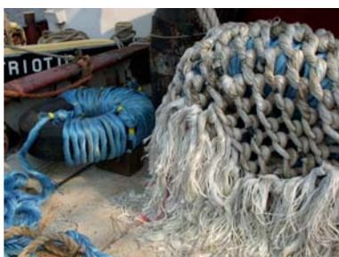
To make these fenders, tires are packed with rope, then served, or wrapped with rope, then “knitted” with half-hitches to make a big “purse.” Finally the whole thing is “whiskered.” The whiskers are made of short pieces of strand that are attached to the knitted hitches.
